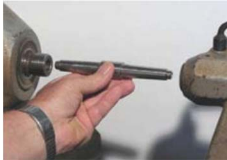
Figure 2. Using the Acruline System to check alignment.
