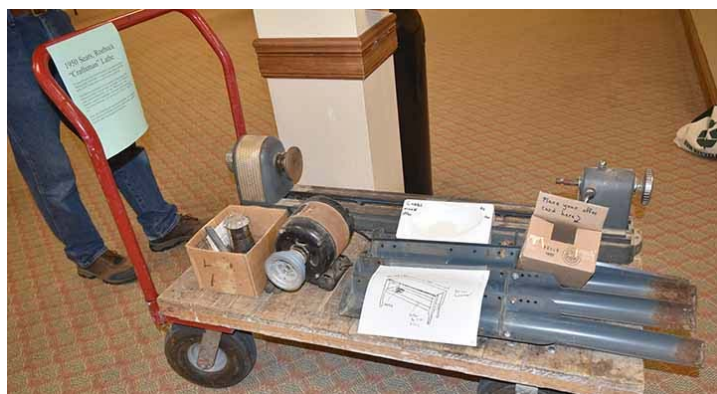
Here's a 50's Craftsman lathe, operable but needing cleaning up.
