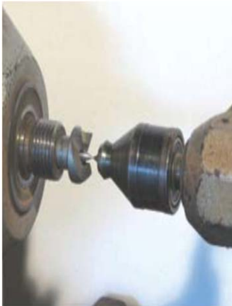
Figure 1. Using two centers to check alignment.
