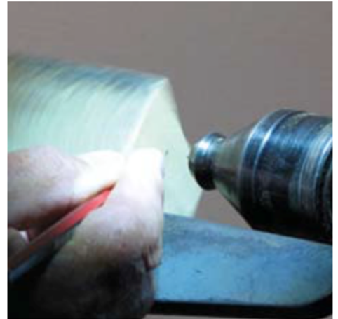
Figure 4. Marking the end of the rotating wood with a pencil.
